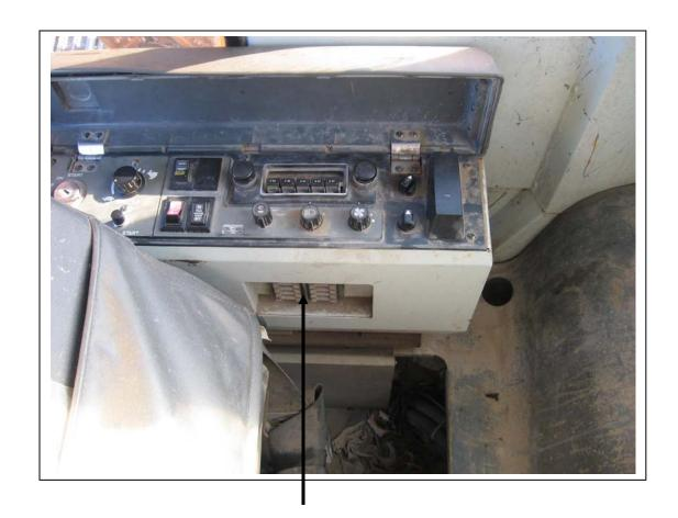
Find power source from back of fuse panel. Ignition live and battery supply.
